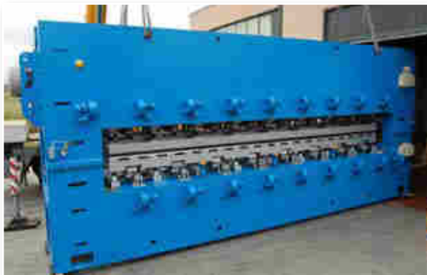
6000 mm Quadropunch con 6000x4 (24000) N/MT 6000 mm Quadropunch with 6000x4 (24000) N/MT
