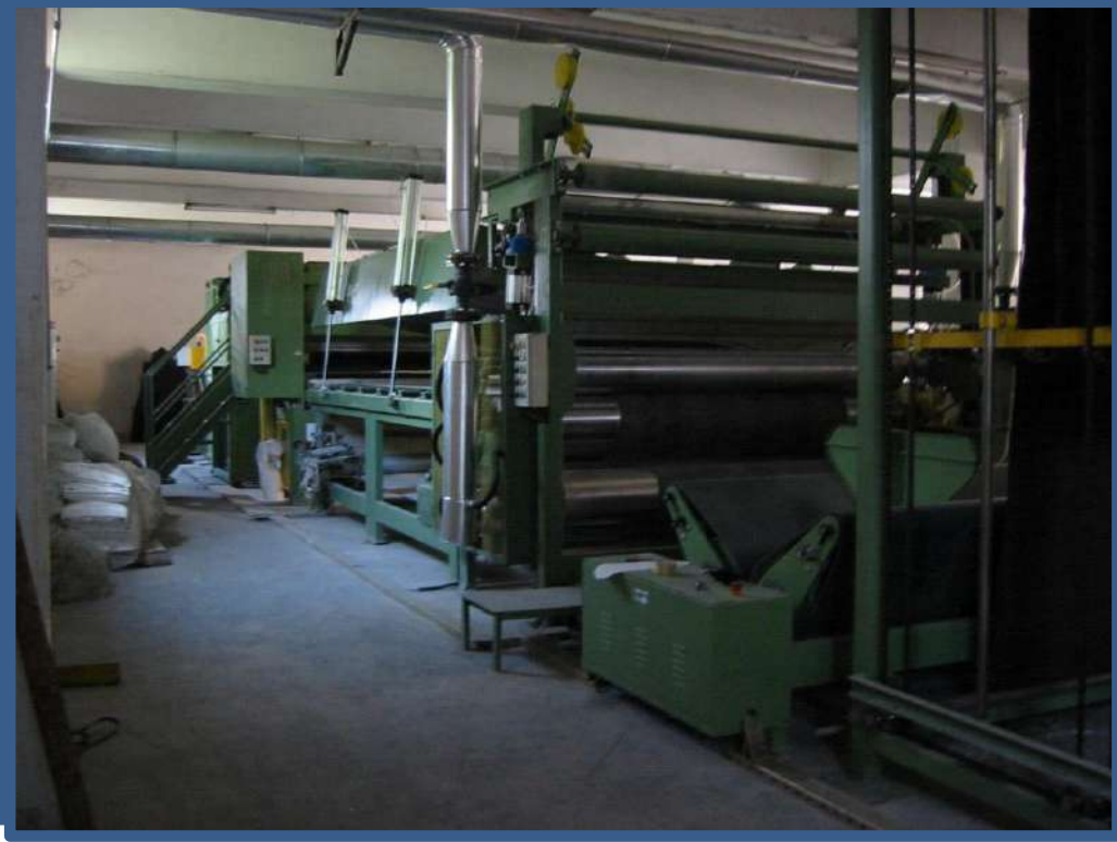
Automotive carpet lamination by powder latex
