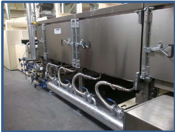
Steam set for the treatment of phenolic powder.
