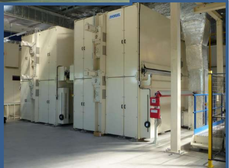
Hydroentanglement and drum dryer in spun lace plant.
