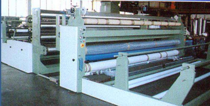
Automotive carpet lamination by powder latex
